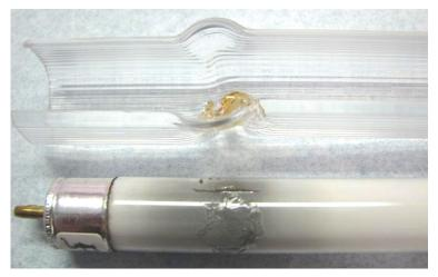
At left is fixture 7F, with the same chipped glass appearance but in addition, an obvious crack in the glass envelope.
