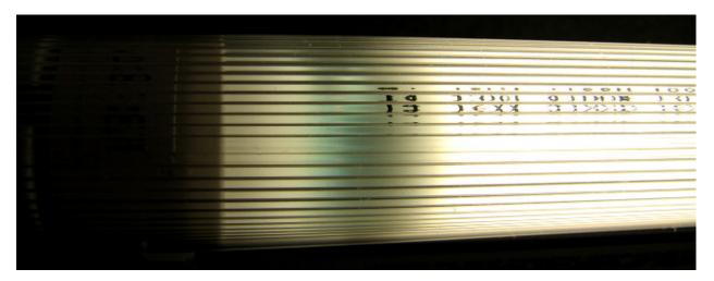
It is unknown what the bluish color signifies, if anything. When tests were first begun on new fixtures, several bulbs exhibited a similar blue or violet glow near the filament but as the end of the tubes darkened, the glow became less visible.
