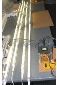
Initially, all twenty fixtures were operated continuously, without power cycling, for 8 hours (pictured at right). The transformer stepped up 120VAC to 240VAC.
