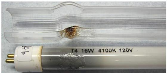
Fixture 7F was found to have been modified at some time by the addition of the same PTC that has been permanently added to all the new fixtures; yet, it's tube still got hot enough to melt the shroud, as seen in the picture above of fixture 7F. The below picture illustrates how the PTC was added to fixture 7F. It is not clear whether this wiring technique is NEC-compliant. However, since the fixtures have plastic cases, there is no danger of this wiring technique shorting.
