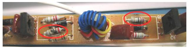
In this case, it appears that the two multivibrator transistors either overheated or the high AC input voltage exceeded their voltage ratings. One of the transistors failed internally, causing its
