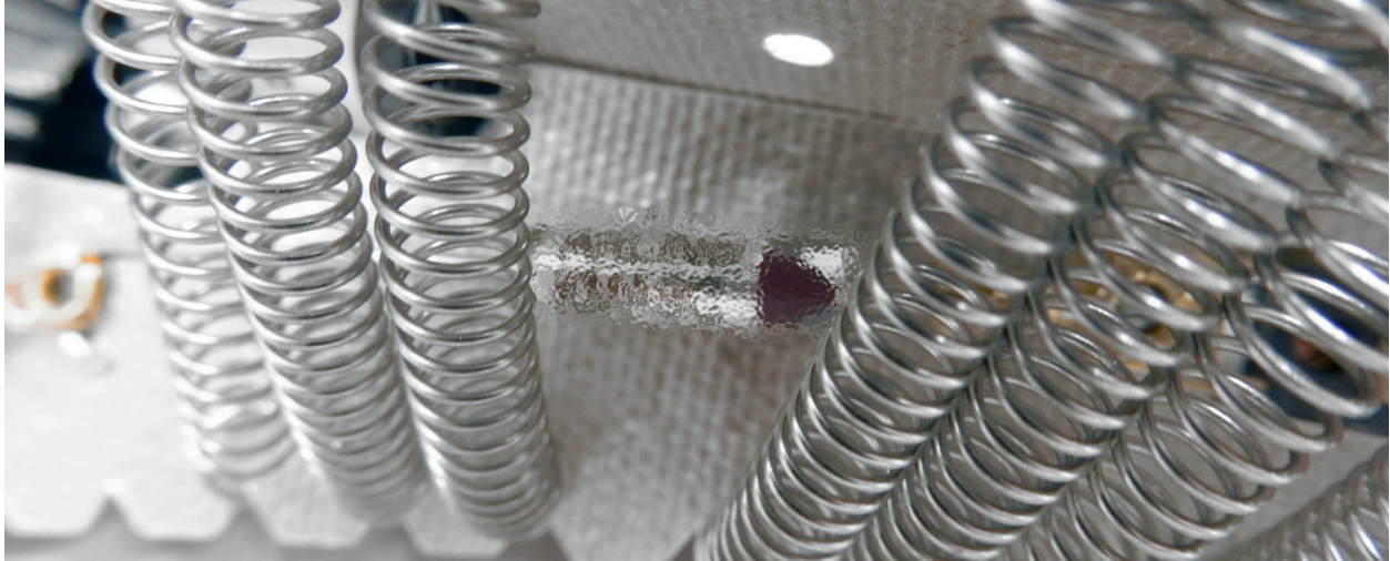
Figure 2: An Brand thermal fuse located within heating element windings
