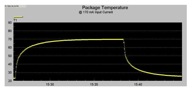
The case temperature can be predicted mathematically by noting that the thermal resistance of the part's SO-8 package is 160°C per watt.
