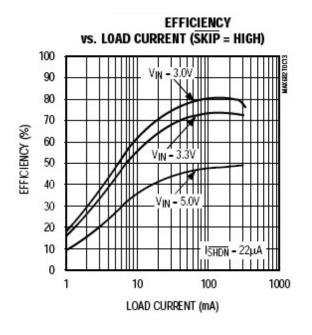
The high temperatures measured and plotted above turns out to be worst-case, because the part actually becomes MORE efficient as the battery voltage drops, as seen in this plot (right) taken from the part specification sheet:
