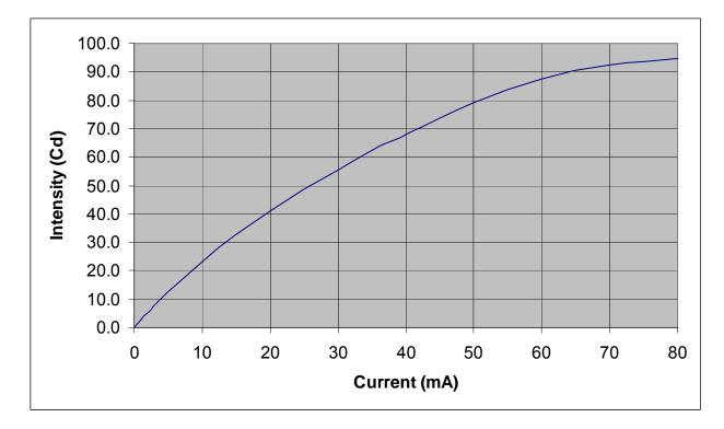
In the client's new-design, the white LEDs are each operating at 20 milliamperes (mA), and so, according to the chart, should be emitting about 40 candelas.
