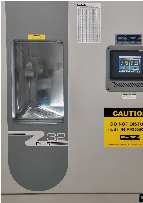
Figure 5: Lamp placed within environmental chamber
