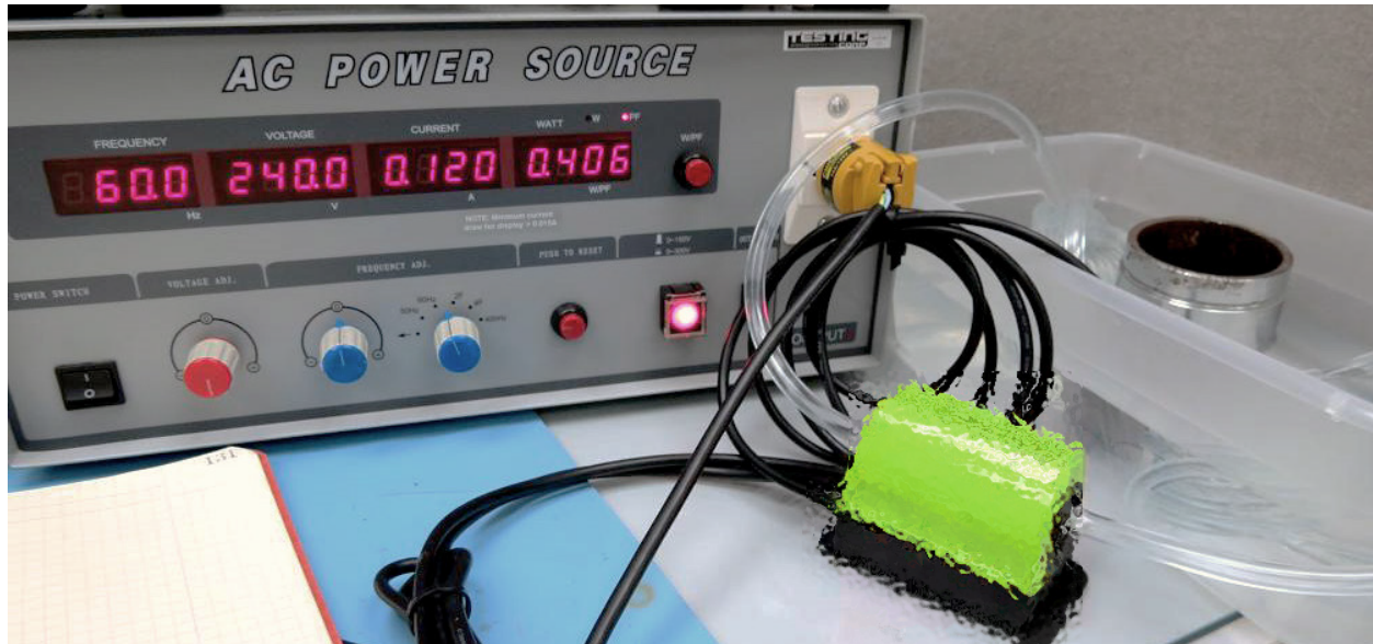
Figure 3: A “New” P-1-Small pump under test at 240VAC. Current of the Small pumps tended to fluctuate somewhat; the current observed after several minutes was recorded below in Table 1.
